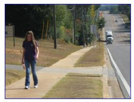
Add Sidewalks For all remaining segments, which represent 84% of the mileage on the study network, the addition of sidewalks (or filling any sidewalk gaps) is recommended. Within this category of recommended sidewalks, three separate unit costs have been developed based on the roadside profile: one for minor re-grading (roadside profile of 1, with 11% of the network mileage), one for major re-grading (roadside profile of 2, with 8% of
